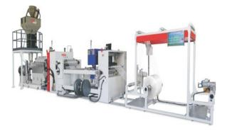
LAMiNA - Mono & multilayer sheet lines for PP/EVA/PS
