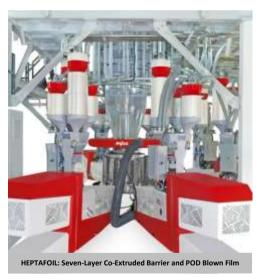
for both symmetrical and asymmetrical structures, with a capacity that will hold the visitors to the booth in awe - 450 kg/hr of film! The line is full loaded with world-class automation — multicomponent batch blending, gsm control,
