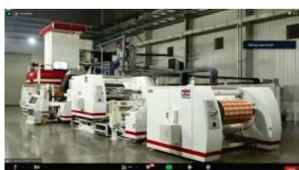
Rajoo-Kohli Lamex 360 coextrusion laminator at Balaji Multiflex in Rajkot Screenshot PSA
